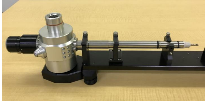
大気非開放冷却二軸ホルダ (Mel-Build製 Double-Tilt LN2 Atoms Defend-Holder)
